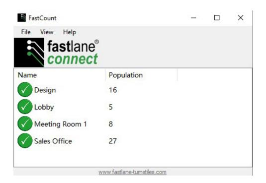
Using Fastlane *Connect*, The TCP/IP communications interface embedded into selected Fastlane and Door Detective products, Fastcount communicates on the same local area network receiving live count information from your selected devices and will allow count information to be supplied from several separate zones configurable on setup.
