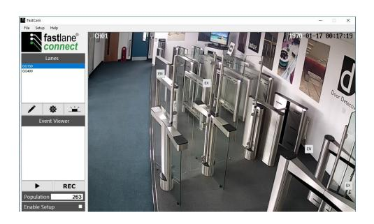
Unique to Fastcam is the ability to add command buttons to the live image stream to enable authorised users to operate the Fastlane turnstiles from their display and keyboard. Options allow the operator to open the lanes in the egress or ingress directions to let a single person enter or exit. Fastcam uses Fastlane *Connect*, the TCP/IP communications interface embedded within most Fastlane and Door Detective products.
